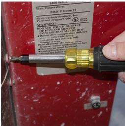
2. Remove the screws from the left side of the box. Skutt kilns have a hinged box which is held closed by 3-6 phillips screws depending on the model.
