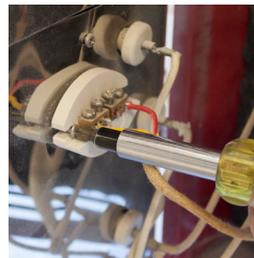
10. Replace the two screws that hold the thermocouple block to the kiln. You didn't lose them, did you?
