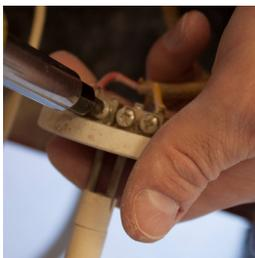
5. Loosen the two center screws on the block that are holding the thermocouple. You do NOT need to take the screws all the way out.
