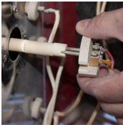
4. Slide the thermocouple out of the kiln. The porcelain block is still attached at this point.
