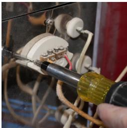
3. Remove the two screws from the sides of the white porcelain thermocouple block. You can follow the yellow wire from the heat baffle to the block.
