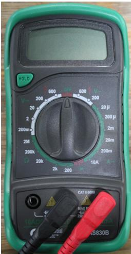
2. Set your electrical meter to "AC Voltage." If your meter does not have an auto range feature you should set your meter to the highest available voltage setting (usually 600 volts). For more information about meters check the PDFs available under the "Learn" tab at kilnparts.com
