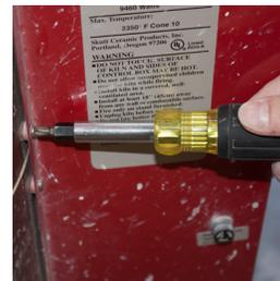
7. Remove the screws from the left side of the box. Skutt kilns have a hinged box which is held closed by 3-6 philips screws depending on the model.
