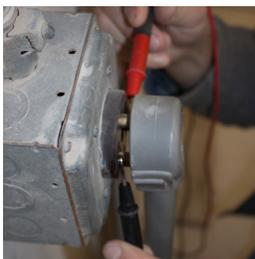
3. Carefully put one probe onto each of the flat blades making sure not to touch anything with the metal probe except the flat metal blade. When testing AC
