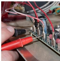
4. With the kiln plugged in, test the voltage between the metal tabs labeled "AC1" and "AC2." You should get 24 Volts (+/- 5%). Note your voltage.
